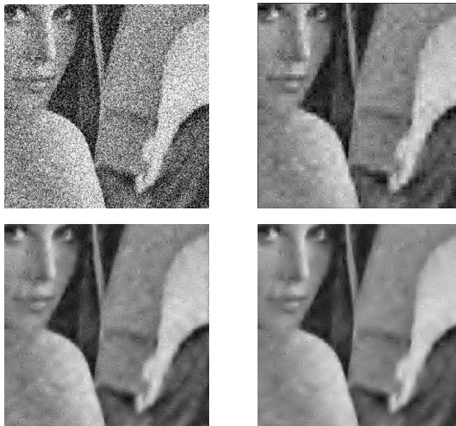
Fig. 7.1 Denoising with frames. Top left: Lena with 34.0dB white Gaussian noise. Top right: Denoised Lena with 25.4 dB noise, using a soft threshold in a single basis. Bottom left: Denoised Lena with 24.2 dB noise, using cycle spinning (frame) from [53]. Bottom right: Denoised Lena with 23.2 dB noise, using differential cycle spinning (frame). The technique used here is an extension of the work in [87] (figure courtesy of Vivek Goyal).
