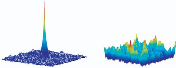
**Fig. 1.** Left: an authentic correlation plane output. Right: an imposter correlation plane output.
