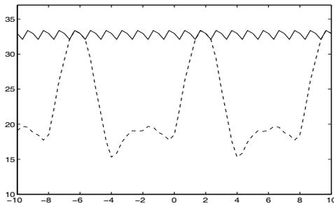
**Fig. 5.** PCE values for a range of possible horizontal shifts for a sample authentic image. A continuous line is used for the WPCF with pre-filtering, and a dashed line for the WPCF without pre-filtering.
