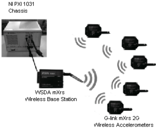
Figure 5. Data acquisition equipment
