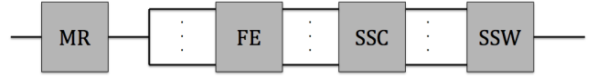
Fig. 3: Semi-supervised MRC. Classification and weighting algorithm in Figure 2 are replaced with their semi-supervised versions so that unlabeled data can contribute to classification.
