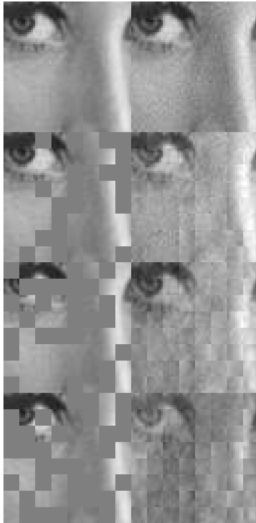
Fig. 2. Results for frame method at 1 bpp. Left column: baseline system; right column: MD system. From top to bottom, number of packets received is 8, 7, 6, and 5.
