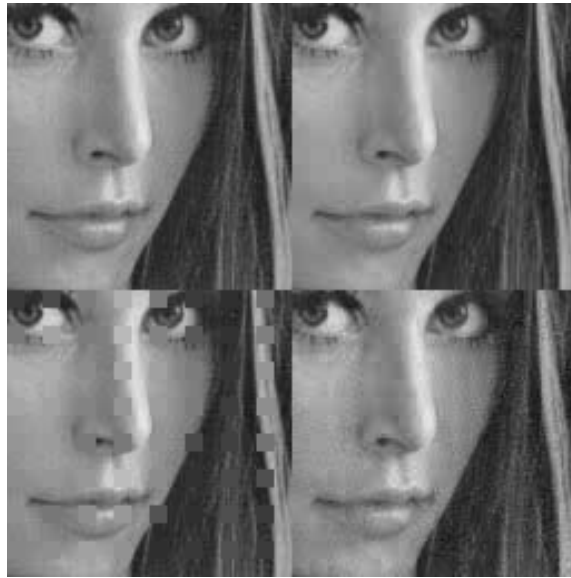
Fig. 1. Results for correlating transform method at 1 bpp. Top row: no packet losses; bottom row: one packet lost. Left column: baseline system; right column: MD system.
