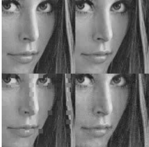
Figure 3: Results for correlating transform method at 1 bpp. Top row: no packet losses; bottom row: one packet lost. Left column: baseline system; right column: MD system.
