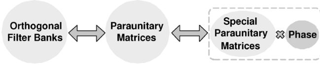
Fig. 1. Relationship among orthogonal filter banks, paraunitary matrices, and special paraunitary matrices: Orthogonal filter banks are characterized by paraunitary matrices in the polyphase domain. Paraunitary matrices are characterized by special paraunitary matrices and phase factors.
